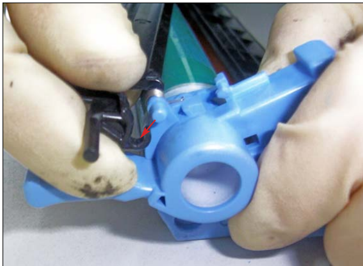
RELEASING THE DRUM SHUTTER FROM THE DRUM UNIT 17. Unhook the drum shutter from its support tab on one side of the drum unit.
