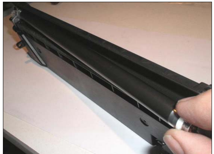
ASSEMBLING THE DEVELOPER ROLLER 66. Reinsert the bushings on each end of the developer roller shown and slide into place.
