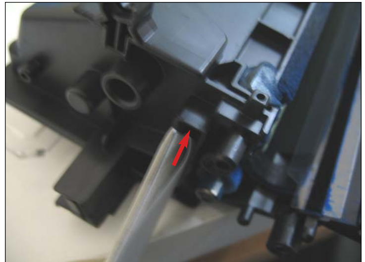
85. Insert the folded tips through the exit seal port opening as shown. Avoid peeling the adhesive backing while inserting the seal.
