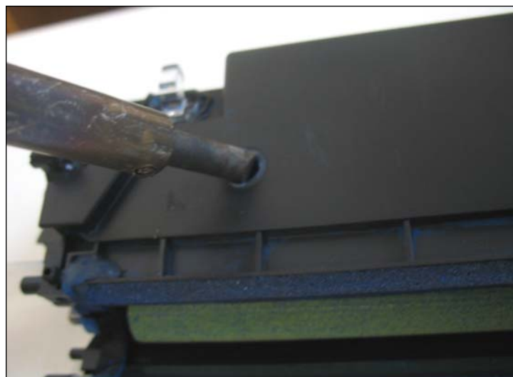
93. Using a soldering tool, melt a small hole through the top of the hopper. This will serve as an opening for refilling the cartridge.
