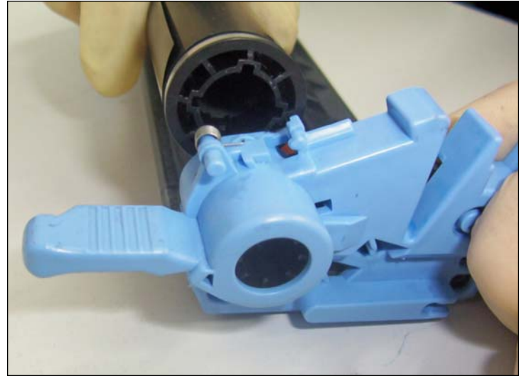
47. Lower the opposite end of the drum into place as shown. Align flange with the axle attachment.
