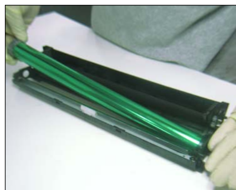
17. Remove the OPC drum as shown.
