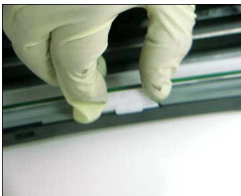
19. Remove the Drum Erase Lamp holder by pulling it off as shown.
