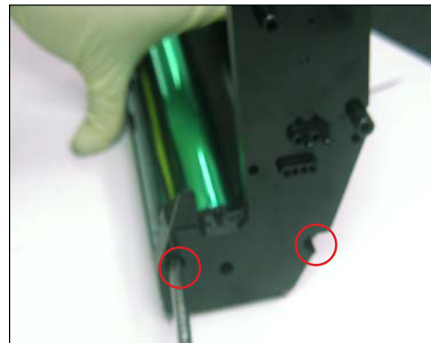
14. Remove the screws on the remaining end cap (gearside) that hold it in place.
