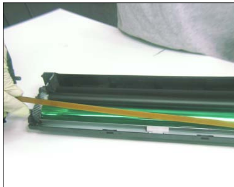
12. Remove the Drum Erase Lamps as shown.
