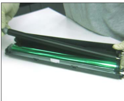
16. Remove the developer roller as shown.
