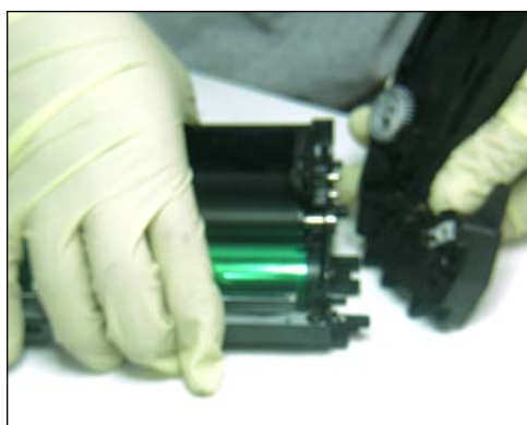
15. Remove the end cap with gears as shown.
