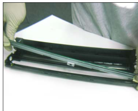
20. Remove the wiper blade as shown.
