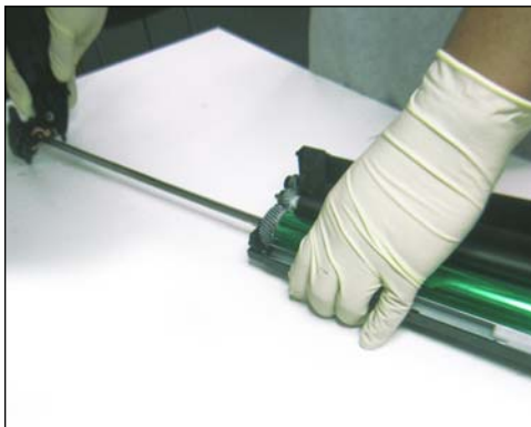
13. Slide the end cap with axle out completely.
