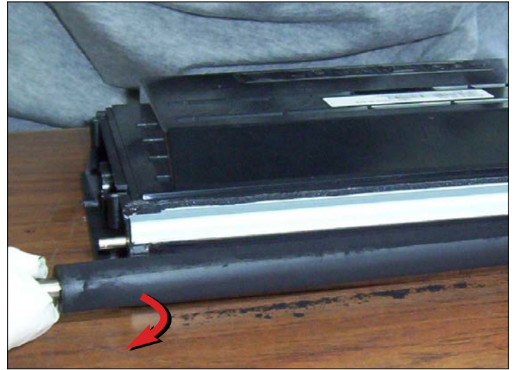
8. Slip the developer roller outward then slide it away toward the side of the cartridge.
