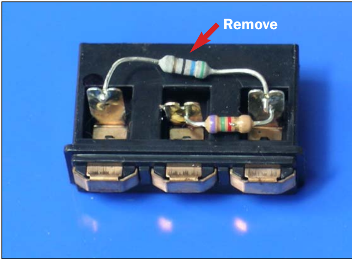
12. Locate the FUSE that is soldered to the two outer contact tabs.
