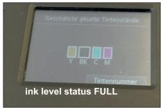
When all refillable cartridges have been set into the printer You can see on the display that each cartrige has been accepted with an full ink level status.
