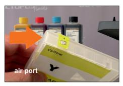
The non-OEM refillable cartridges suitable for Canon's PGI-1500 or PGI-2500 inkjet cartridges have a fill port on their back. This port is closed by a soft silicon plug. On the cartridges' upper side there is the air port. When receiving the refillable cartridges this opening is closed either by a strip of yellow tape or a silicon plug. depending on the production batch.
