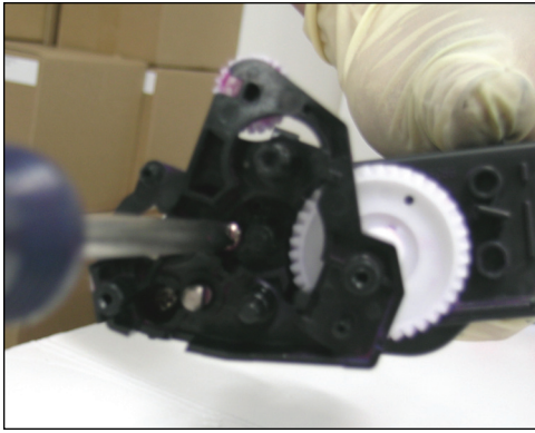
21 Remove two first screw as shown.
