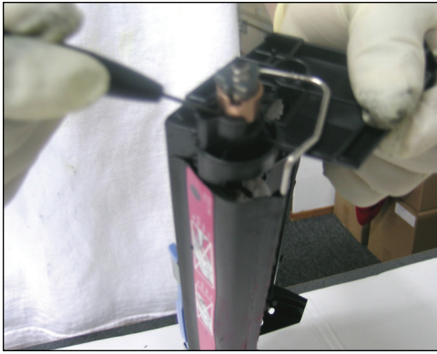
53 Pry out the axle bearing as shown.
