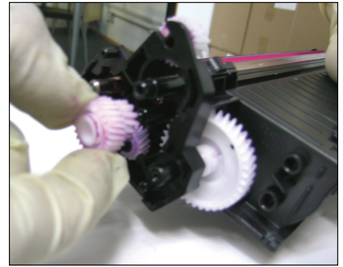
17 Remove first inner-gear as shown.
