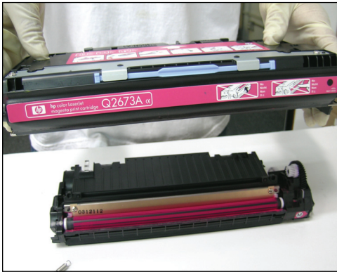
7 Separate the drum unit from the toner cartridge.
