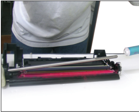
56 Slide out the drum as shown.
