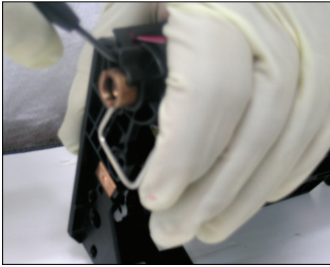
44 Pry off the axle bearing with a small flat screwdriver.
