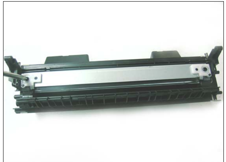
22. Remove the two screws holding the doctor blade to the toner hopper. NOTE: The two screws used to hold the doctor blade are longer than the normal cartridge screws. Make sure the correct screws are used when reassembling the toner hopper.
