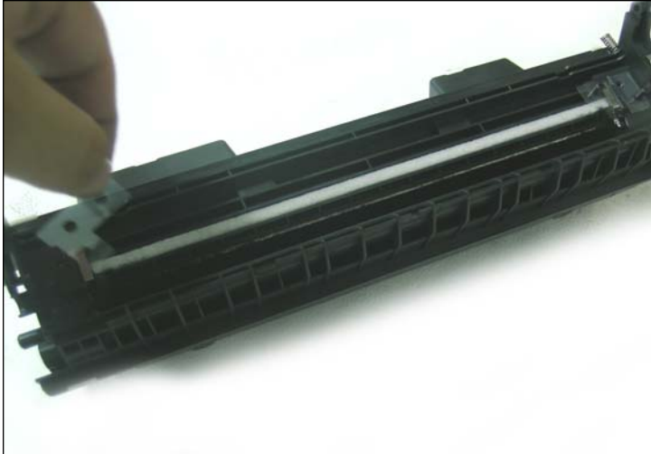
26. Install the two mylar shims that sit under the doctor blade.
