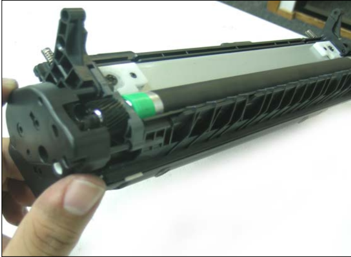
32. Slide the gear housing end cap onto the toner hopper. Install the two screws that hold the end cap to the hopper.
