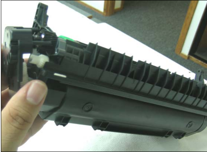
17. Pull the gear housing end cap from the end of toner hopper.
