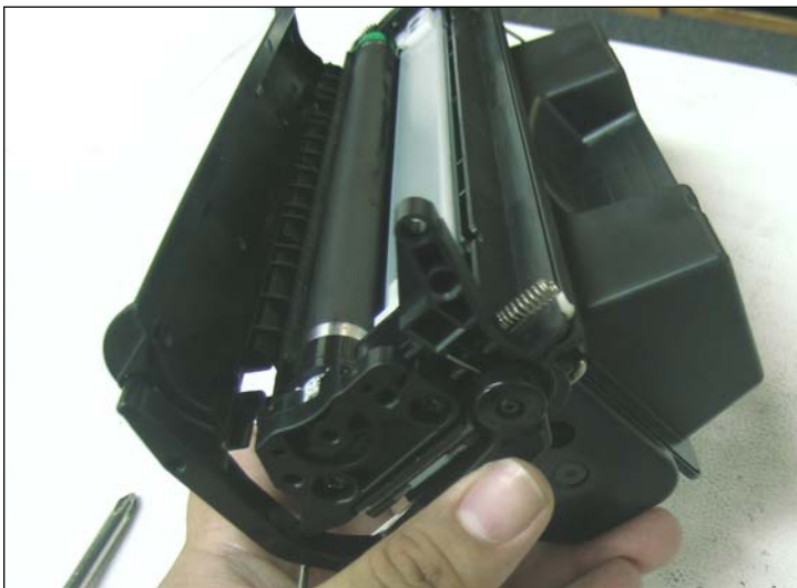
35. Open the shutter to engage the tension spring.
