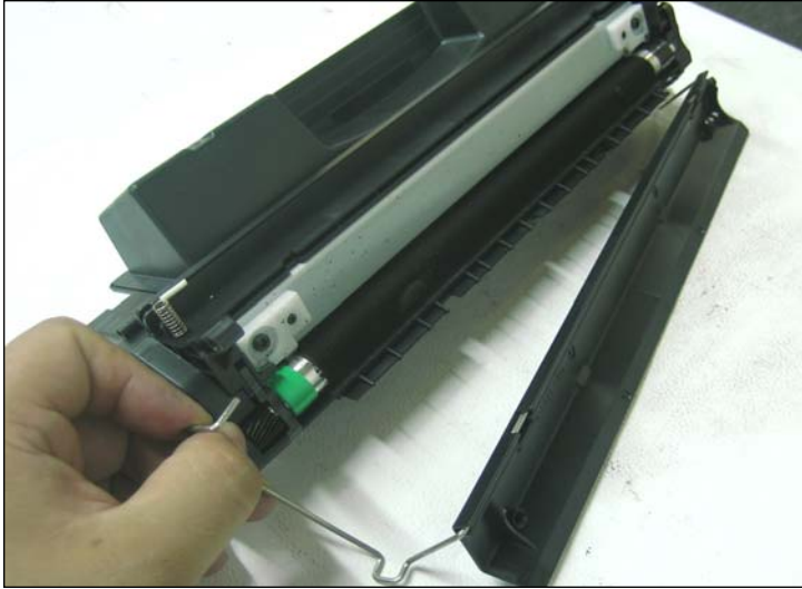
15. Remove the drum shutter bar from each side of the toner hopper and remove the shutter.
