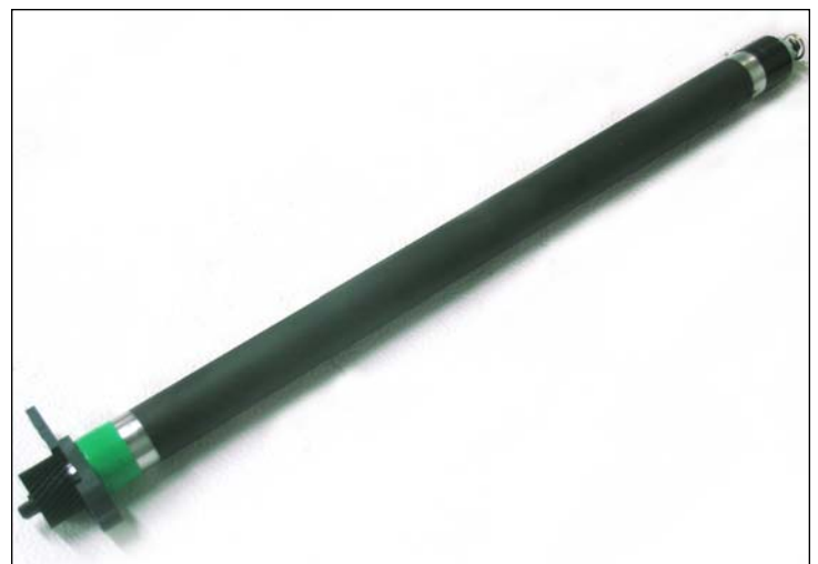
29. Slide the black mag roller bushing onto the contact side of the mag roller, and the green bushing onto the drive gear side of the roller. Install the stabilizing bar onto the mag roller with the C-bear facing towards the mag roller bushing. The mag roller drive gear will fit onto the mag roller either way, however the flat side of the drive gear needs to face the mag roller-stabilizing bar and the side of the gear that has the dimples faces outward.
