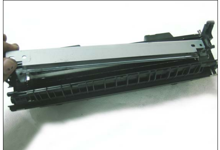
27. Place the doctor blade onto the toner hopper.
