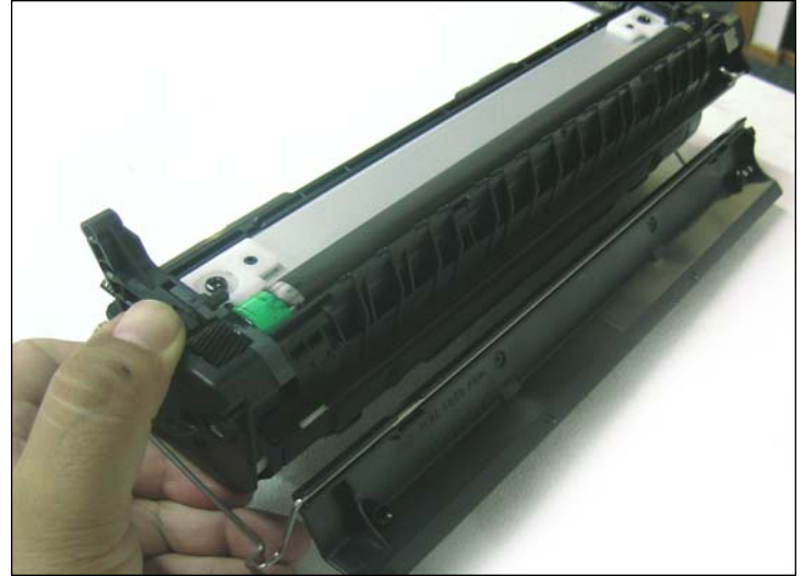
33. Install the drum shutter bar into the slots on each end of the toner hopper.
