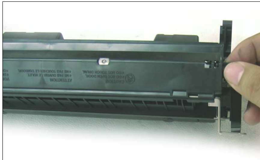
34. Slide the drum shutter arm onto the alignment post and install the shutter arm to the drum shutter.
