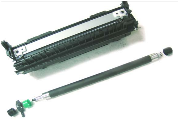
21. Lift the mag roller out from the toner hopper. Remove the black drive gear, the stabilizing bar and the mag roller bushings from the ends of the mag roller. Using dry compressed air or a vacuum, clean the toner off the mag roller. Clean the roller using a lint-free cloth and a mag roller cleaner. Clean the roller bushings should be cleaned using a lint-free cloth and alcohol. NOTE: Do not lose the C-bearing that sits inside the stabilizing bar.
