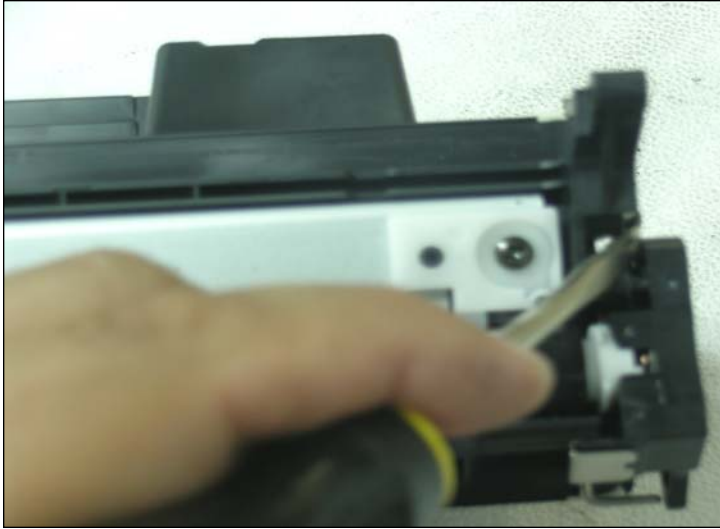
19. Using a small flat blade screwdriver press down on the locking clip that holds the contact end cap to the toner hopper.
