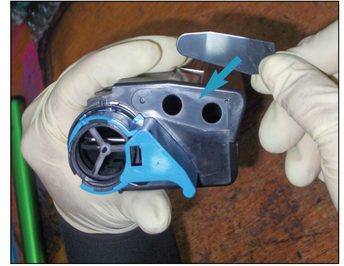
30. After cleaning use alcohol to clean both the cartridge and the tab openings, then reinsert the adhesive tab.
