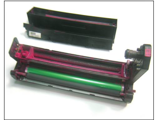
6. The plastic cover and drum unit can now be separated.
