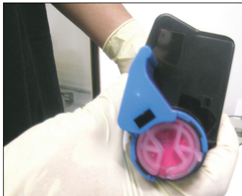
35. White tab lifted. Remanufacturing concluded.
