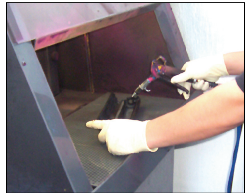
24. Clean using air pressure. Reassemble when done.
