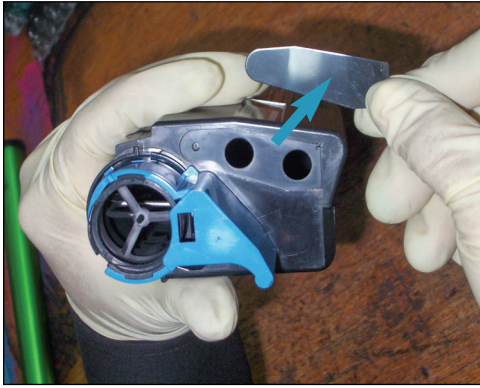
28. Using a thin needle or small hook tool, pry off the plastic adhesive tab from the waste hopper openings (two holes) shown. This is where the waste toner will dump out during cleaning.
