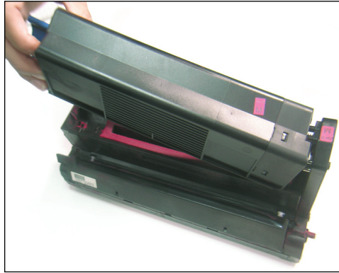
2. Remove toner unit and set aside.
