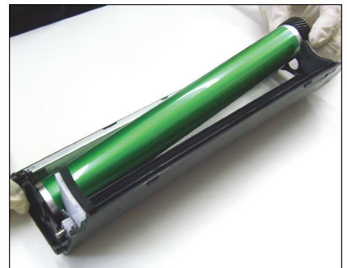
18. Carefully remove the cylinder as shown gear-side first.
