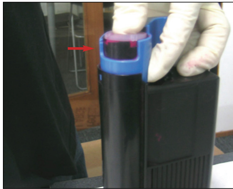
32. Radial plug by making sure the tab lines up with the slot.
