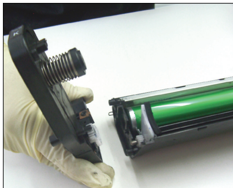
17. The large end cap should easily come out.
