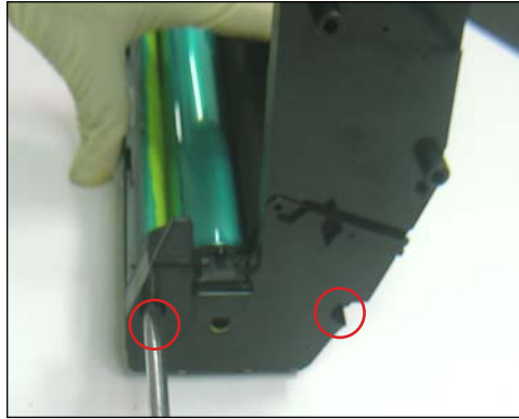
13. Remove the screws on the remaining end cap (gearside) that hold it in place.
