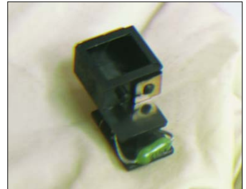
20. After cleaning and refilling the cartridge, replace the fuse and reassemble the cartridge by following the steps in reverse order.
