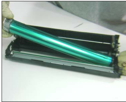
16. Remove the OPC drum as shown.
