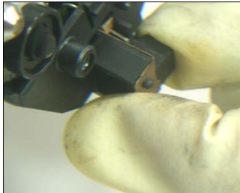
19. Pull out the fuse holder located on the side of the cartridge.
