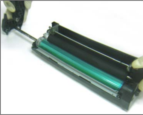
12. Slide the end cap with axle out completely.
