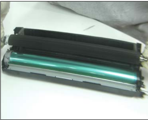
15. Remove the developer roller as shown.
