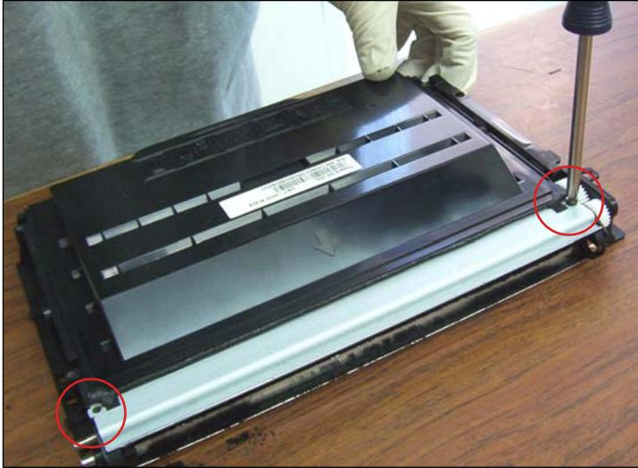
**9. Remove the metal cover where the sealing blade is located by unscrewing two screws located on the top of the cartridge.**
