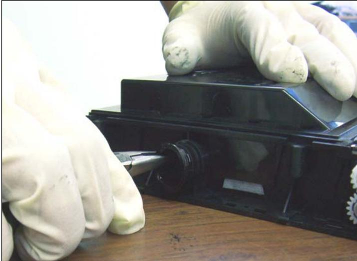
**11. Remove the toner fill plug and start the cleaning process. Use a vacuum on easy areas making sure there is nothing that will vent. Use air pressure for hard-to-reach and sensitive areas.**
