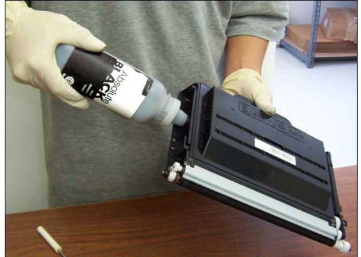
**12. After thoroughly cleaning the cartridge and reinstalling cleaned components, you are ready to install your after-market toner.**
