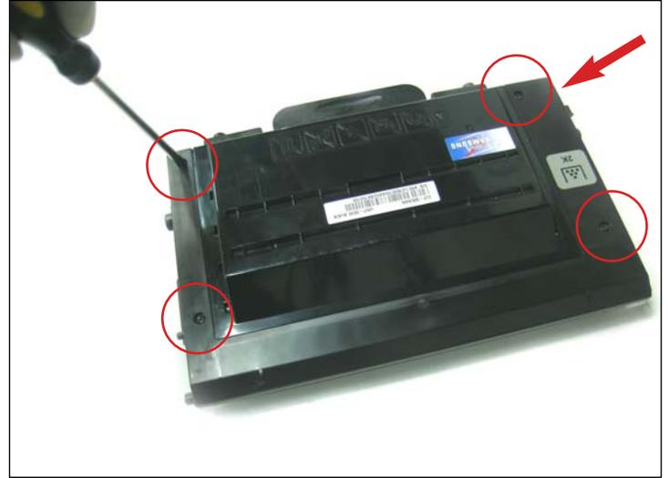
**1. Remove the four screws located on the top and the fifth near the gear side of the outer shell as shown.**
