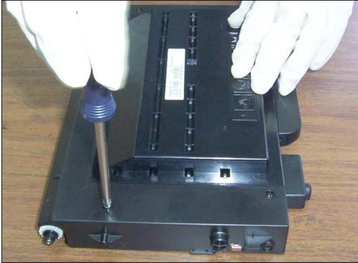
1. First, remove the outer shell by loosening and removing five screws. Four are located on top of the cartridge.
