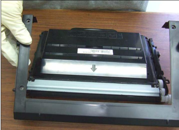
3. Remove the cover as shown. You will notice a small adhesive holding it in place, but it will not be affected if the cover is removed.
