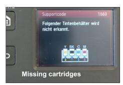
On the display is shown that no cartridges are in the printer (we removed all the cartridges before). With that status the print head moves to the exchange position automatically when opening the printer's front cover. Now You can install the missing cartridges using the printer's support.
