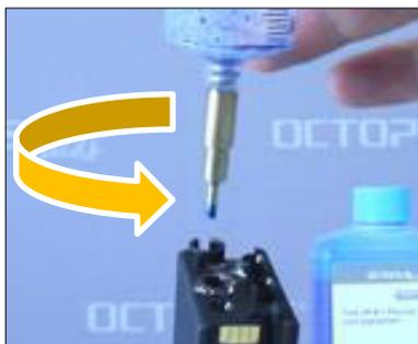
Remove the QU-Fill™ refill tool from the ink outlet. We recommend turning it slowly. This avoids that the rubber fitting inside the ink outlet will be dislocated. If it should occur that the fitting slides out of its position, You can push it back carefully.
