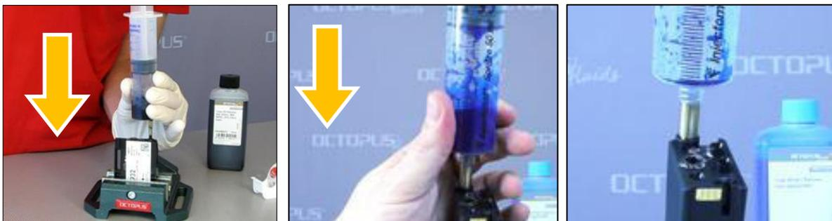
Release the plunger and it will slide back autonomously. It is not necessary to push the plunger or press the ink into the cartridge. The refill ink flows into the cartridge by itself and compensates the negative pressure inside. Repeat the procedure several times until no air bubbles arise anymore when pulling the plunger upwards and / or the wanted quantity of refill ink has been filled completely into the cartridge.
