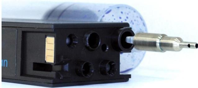
The QU-FILL™ *professional* refill tool enables You to refill HP 950, 951, HP 932, 933 and HP 970, 971 inkjet cartridges without further modifications of the cartridge. A few preparing steps and You open the spring valve in the ink outlet by using the QU-FILL™ *professional* refill tool, You create negative pressure in the inside of the cartridge and the refill ink is sucked into the cartridge out of the refill syringe.
