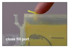
For filling the non-OEM inkjet cartridges suitable for Epson® 27, 27XL take out the plug from the fill port and keep it for later use. The suitable quantity of refill ink for these refillable cartridges is **9 ml to 10 ml** pigmented refill ink. Best printing results can be accomplished by using dedicated refill inks whose physical characteristics have been adjusted to the original Epson 27, 27XL inkjet cartridges.
